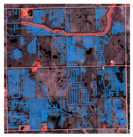
Figure 3. Example of a drainage network beneath cropland.
